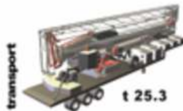
transport crane and complete ballast on 1 truck gru e zavorra completa su 1 camion
